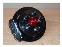
Various Different versions of the brake kit can be used, options include rotor size, caliper style, and colours, or polished finishes
