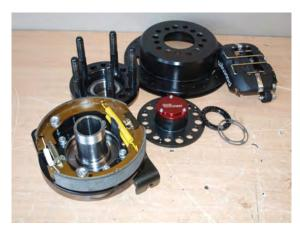
We also supply our flanged spindles, spacer brackets, and all hardware to mount the Wilwood brakes
