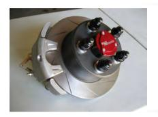
Our RPB050/051 Brake kit is a street legal brake kit using Falcon calipers, and 279mm DBA rotors. 180mm from wheel mounting face to inner most point of caliper
